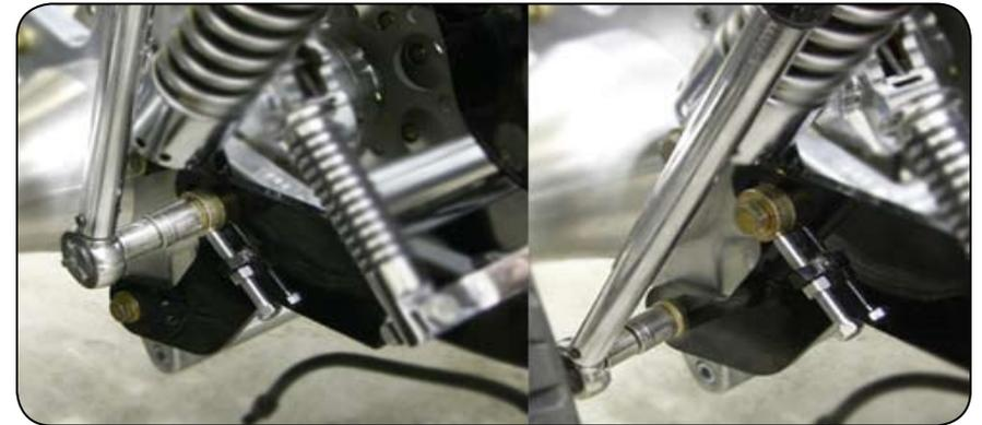
18. Hook up stock brake line, bled rear brake, tighten lug nuts on rear wheels torque 78 to 85 ft. lbs. and go for a ride. Re-torque lug nuts after 25 miles or 100 mile maximum.
