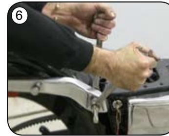
6. On '91-'05 Install shock studs, use nut from original shock studs. 06' and UP use your shock stud. **Use blue loctite.**
