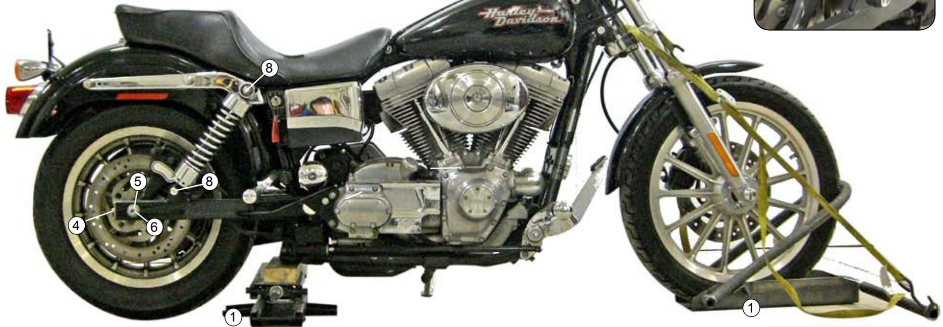
9. Remove the banjo bolt from caliper
