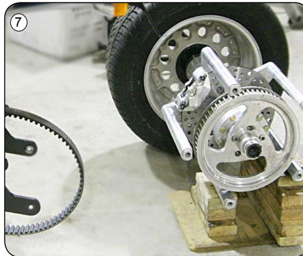
8. Slide the rear end under the bike. Lower the jack and set belt on pulley. (This is a little tricky but have patience) This is shown with a 65 tooth pulley. For larger pulley you may need to loosen the spokes on the opposite side of rear end to accomodate the belt installation. You may have to work around each spoke spreading then inserting belt while lifting the axel.
