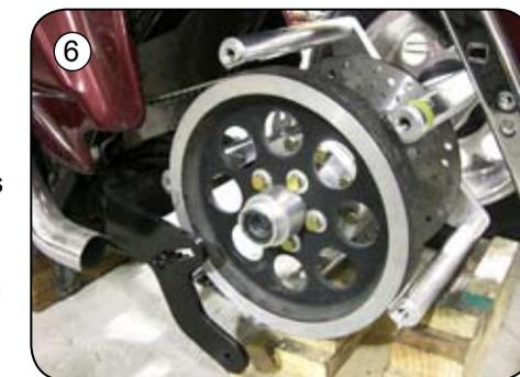
8. Slide drive side star plate onto rear end differential housing, align the star plate with the spoke that was marked with the green tape. Start all 1/2" allen bolts on star plate into spokes, tighten evenly. **DO NOT FORCE BOLTS IN**
