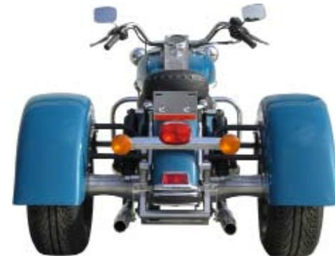
Our Trike rear ends are made from all 6061 T6 billet aluminum, except for our Sport Trike rear end, which has 3/8" thick steel star plates, powder coated silver, instead of 1" thick billet aluminum star plates that we use on all our other Trike rear ends.
