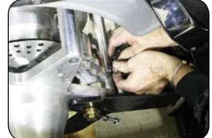
**⚠** The trike must be sitting on the ground on its suspension to adjust the belt. Shown without wheel and on blocks for photography.
