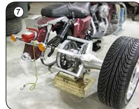
7. Slide the rear end under the bike. Lower the jack and set belt on pulley. (This is a little tricky but have patience) This is shown with a 65 tooth pulley. For larger pulley you may need to loosen the spokes on the opposite side of rear end to accommodate the belt installation. You may have to work around each spoke loosening spreading then inserting belt while lifting the axel.
