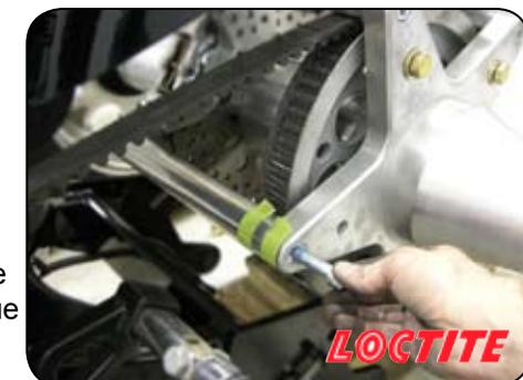
9. Remove the 1/2" allens one at a time apply blue loctite and reinstall torque 60 ft. lbs. Both Sides.
