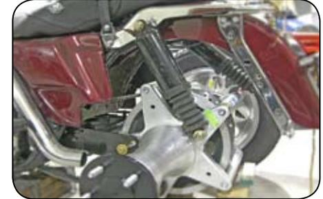
13. Install brake line to rear caliper and bled.
