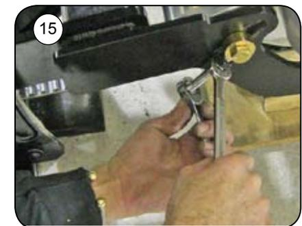
**⚠** *The trike must be sitting on the ground on its suspension to adjust the belt. Shown without wheel and on blocks for photography.*
