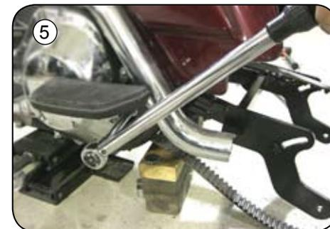
6. Prepare a Block and position rear end as shown to the right.
