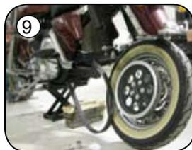
10. Lower the bike down, place wood blocks under the transmission to support the transmission for removal of the swing arm.
